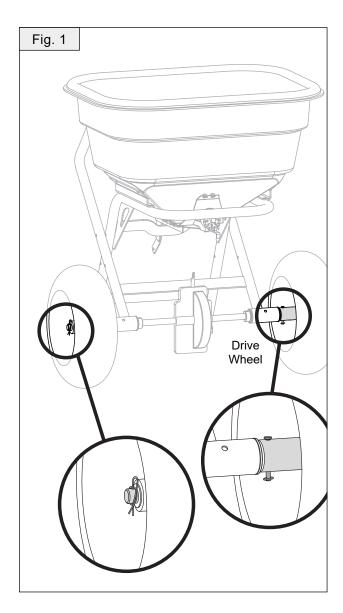
1b. Install Wheel on each side of axle (Valve Stem Out). On the drive wheel side, install 3/16 x 1-3/4" Clevis Pin and Cotter Ring, Figure 1. On opposite side install wheel washer and Rue Ring Locking Pin on outside of wheel.
