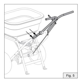
6a. Install two agitator wires on the upper spinner shaft.
