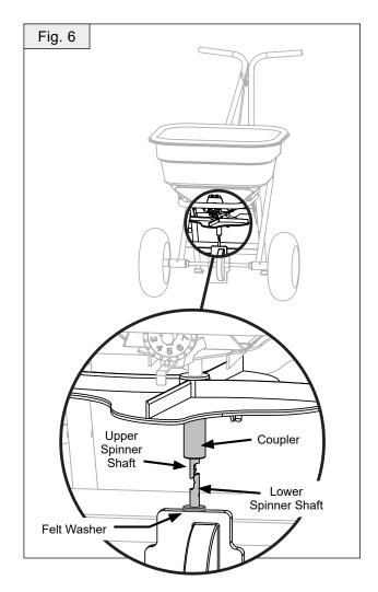
6b. Install felt washer on shaft below the agitator wires. Slide shaft down through hopper. Install the fan and coupler, *see Figure 6*.
