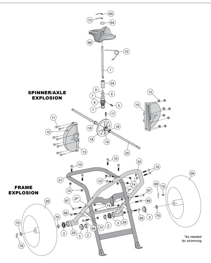
1a. Remove clips from axles on the outside of axle frame assembly.
