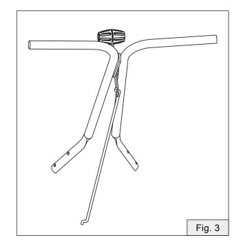
4. Turn handle/linkage assembly sideways and insert end of linkage into rate gate linkage, Figure 4.
